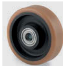
Wheel: STP 92 Shore A Wheel centre: pressed steel, welded, lacquered, Tread: Polyurethane, casted, precision ball bearing
