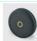
Wheel: XGI electric conductive Wheel centre: Polyamide, Tread: TENTEprene (thermoplastic rubber), plain bearing
