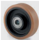
Wheel: FTP 92 Shore A Wheel centre: Steel, lacquered, Tread: Polyurethane, casted, precision ball bearing
